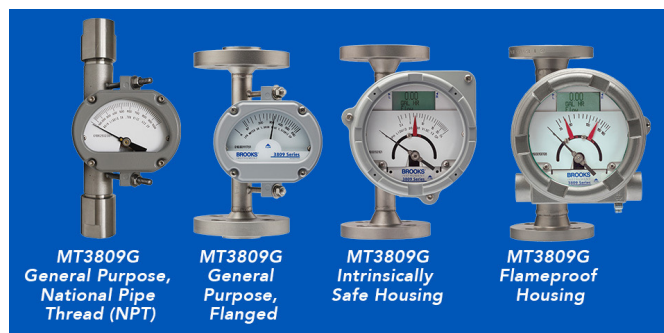
Figure 1. Variable area flowmeters like the MT3809G from Brooks Instrument are durable and accurate for high-pressure and extreme temperature applications. For offshore applications, well-constructed VA flowmeters typically use 316/316L Dual Certified stainless steel with Alloy 625, Hastelloy C-276 or Titanium GR II.
